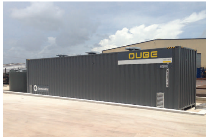
CleanaWater Multi-purpose Water Recycling System in 40ft Shipping Container
